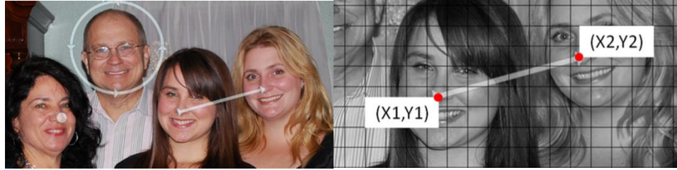
Figure 2. Illustration of picture password on Windows 8. On the left are the common gestures and on the right are the recorded coordinates used for authentication. (Courtesy of MSDN Blog 2 )
